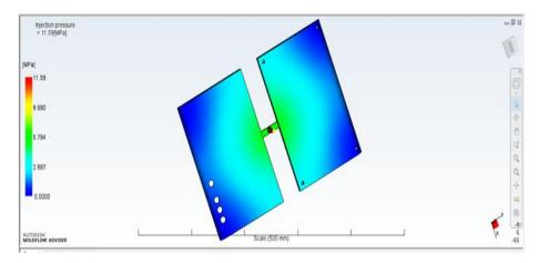
Fig. 9 InjectionPressuredistribution
