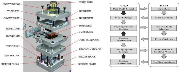
Fig.1 Standard Two PlateMould
