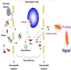
Figure no. 4: Mechanism of Glucose Biosensor
