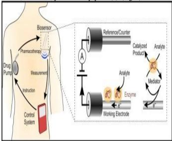
Figure no. 2: Implantable electrochemical biosensors
