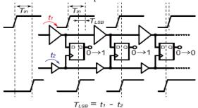
Fig. 1. Simplified schematic of a typical Venire TDC.
