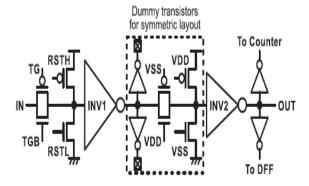
Fig. 6. Detailed schematic of the PSB.
