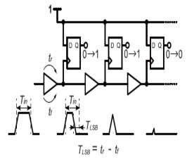
Fig. 2. Simplified schematic of a typical PS TDC.
