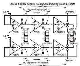
N to 2N-1 buffer outputs are fixed to 1 during stand-by state
