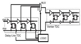
Fig. 4. Schematic of a typical TS TDC [14], [15].
