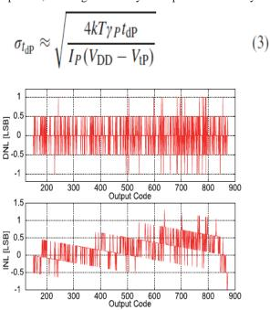
Fig. 16. Simulation results of DNL and INL of the fine-stage PS TDC.
