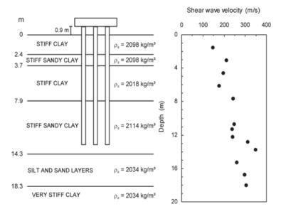
Fig. 5: Layout of pile group, soil profile and soil properties
