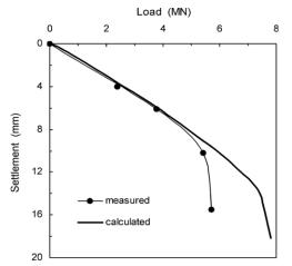
Fig. 4: Comparison of measured and predicted load-settlement behaviour for pile group- o'neill (1981)
