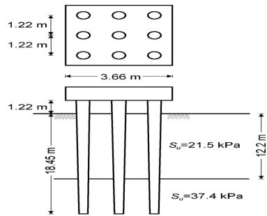
Fig. 3: Schematic diagram of pile system
