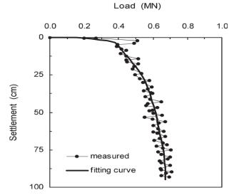
Fig. 12. Load-settlement response of single pile with indication of fitting curve - conte et al.(2003)
