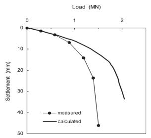
Fig. 2: Comparison of measured and predicted load-settlement behaviour for pile group-koizumi and ito (1967)
