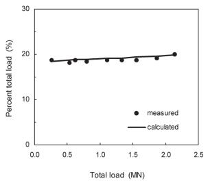
Fig. 10. Comparison of the calculated and predicted loads carried by the central piles -briaud et al. (1989)
