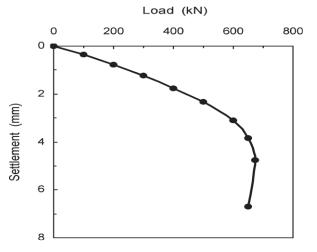
Fig. 6: Average load-settlement curve of the isolated piles- o'neill et al. (1982)
