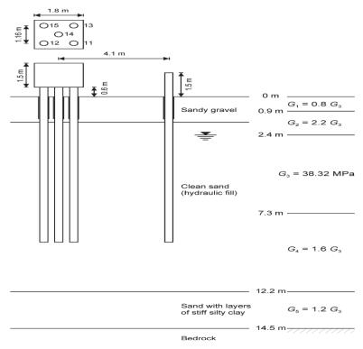
Fig. 8. Layout of the pile group and soil profile- briaud et al. (1989)
