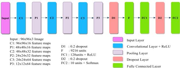
Fig. 1.: Architecture of the proposed fish species underwater image classification model.
