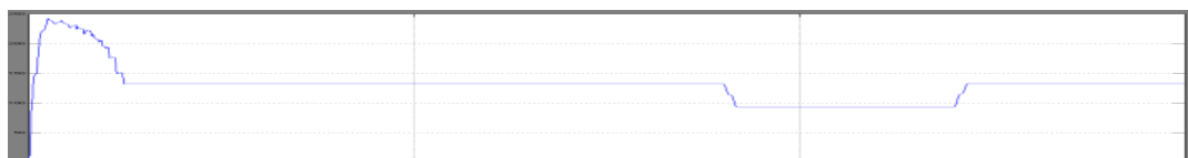
Fig.15. RMS value of source voltage during sag
