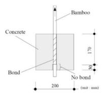
Figure 4: Typical Pullout test for Bamboo [8]
