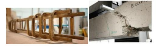
Figure 5: A typical bamboo reinforcement & failure of a bamboo concrete beam [Alireza Javadian, 26]
