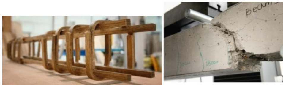
Figure 5: A typical bamboo reinforcement & failure of a bamboo concrete beam [Alireza Javadian, 26]
