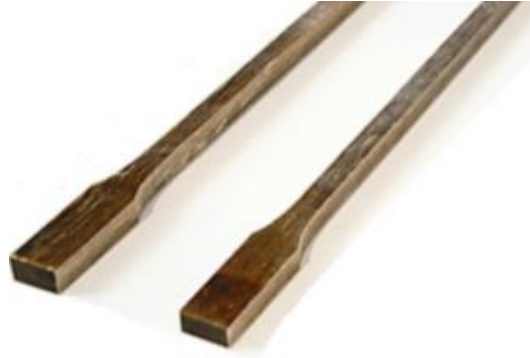
Figure 6: A typical bamboo tensile test specimen [Alireza Javadian, 26]
