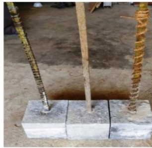
Figure 7: Specimen for reinforcement pull-out test [2]
