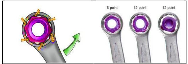
In comparison with an open-ended spanner, the ring spanners are less slippery over the fastener, because ring spanners provide large contact points with the fasteners in all possible points. This implies the turning arc will be more with large action and make the task effective and quicker.
