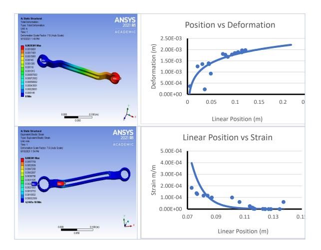
**Conclusion:** In this design and analysis, the result shows that chrome vanadium steel offered a small deformation around 2.03E-3 m; when fixed the bid end with the surface condition as a remote force of 500N. The maximum deformation at another end (small ringside). The maximum stress concentration occurs at the offset section, caused the localized stress to develop around 1.249E+9 Pa. Stress distributed exponentially after the offset section and get normalize by the end of the spanner.
