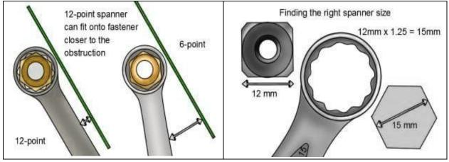
Ring spanner sizes are given as the size of a head of a hexagonal fastener the spanner can be used on. Ring spanner profile sizes are available to fit hexagonal fastener head sizes ranging from 4mm to 50mm or 5/32'' to 2". The spanner length increases with the size of the spanner head, from about 100mm (4") to 500mm (19<sup>1</sup>/<sub>2</sub>").
