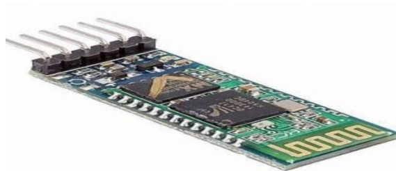
Fig 6. Rf Transceiver Module
