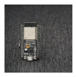
ESP32 Processer is a hybrid microchip which supports Wi-Fi and Bluetooth connectivity for wide range of devices. It's one of the main IoT learning tools. *This* provides full Linux system platform at a very low price with a very robust design and is highly integrated with built in antennas [5].
