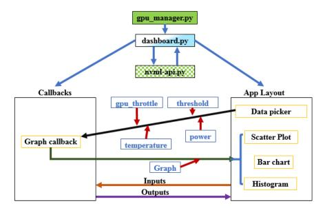
Figure 3: Data flow diagram of GPU Watcher
