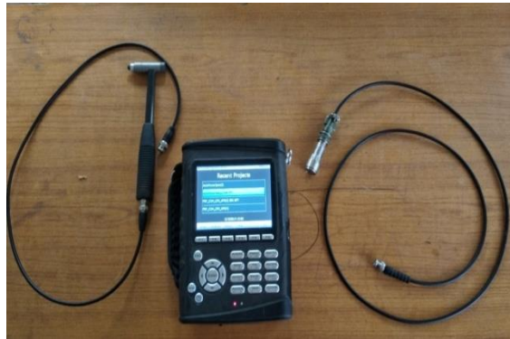
Fig 8 FFT analyser along with impact hammer (on left side) and an accelerometer sensor (on right side).
