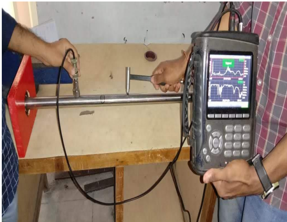
Fig 9 Image of experimentation on the shaft using FFT analyser
