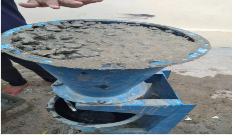
Figure 2.6.2.iii compaction factor test
