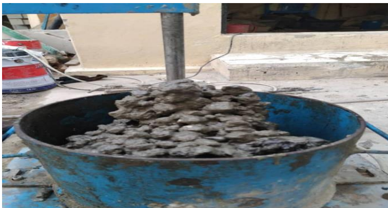
Figure 2.6.2.ii vee bee test
