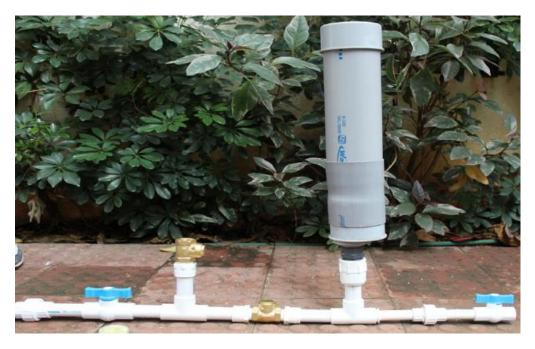
Fig. Completed assembly of the Ram Pump
