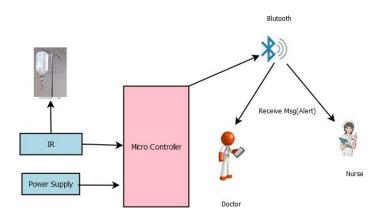
The main objective of system is to provide authentic, accessible, easy and economic system for saline level monitoring. The saline is inserted into blood by considering certain characteristics like heart rate, blood pressure, body temperature, pulse rate and body weight of patient. As the saline goes below the threshold level, it is necessary to change the saline bottle. An automatic saline level monitoring consists of IR sensors which are used to determine the status of liquid in
