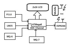
Figure No 1: Hardware components Block Diagram.
