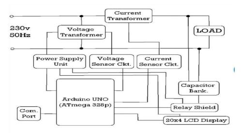
Figure no III Block Dig of IOT Cloud based power factor controller is shown in below fig.
