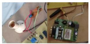
Load connection and GSM module
