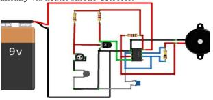
FIGURE: FIRE ALARM SYSTEM
