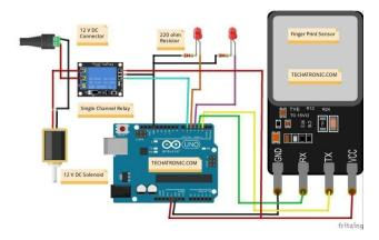
FIGURE: Fingerprint security system
