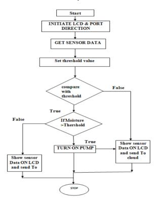
Figure no 6: Flowchart of working of greenhouse using IOT
