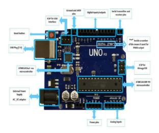
Figure no 7: Microcontroller (Arduino) used for controlling
