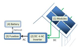
Figure no 3: PV system and storage of solar energy
