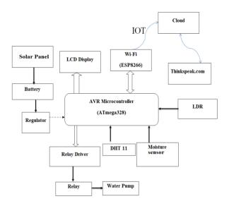
Figure no 5: Working principle of IOT in greenhouse
