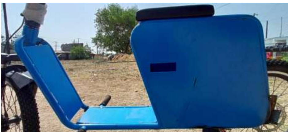
Figure 2: Stand frame for batteries installation
