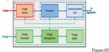
In the IoT system we have a need for ultra-low powered smart sensors along with energy efficient high performance cloud computing devices. The answer is smart sensors will need just enough performance to obtain the input from the sensors, process the signal and send the results to the communications system to be transmitted to the
