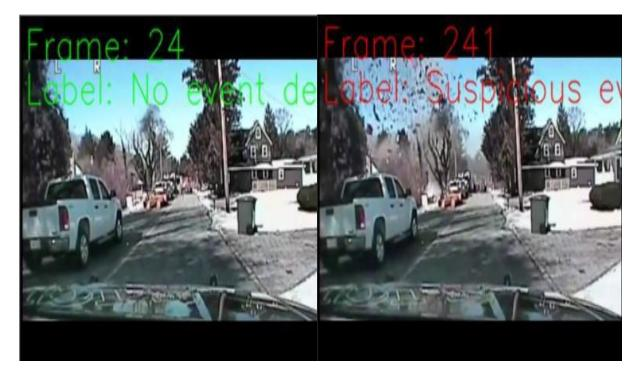
In the figures above, the green color indicates that the activity is not suspicious, while the red color indicates that the activity is suspicious. When a suspicious detection is detected, it will appear on the LCD screen and alert the user.
