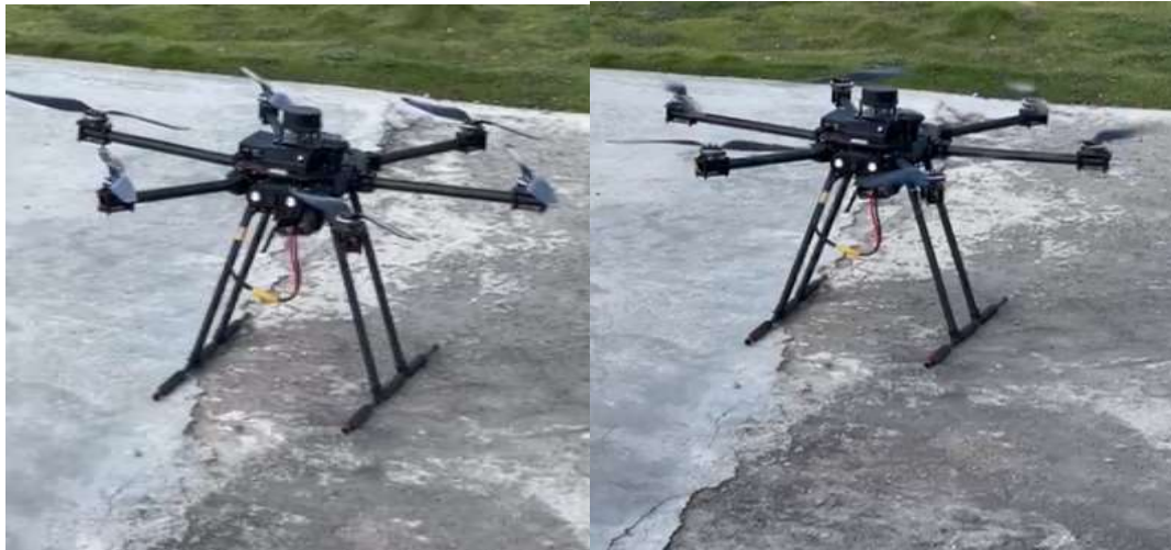
Figure 5: LiDAR integrated Drone with six-propellers.
