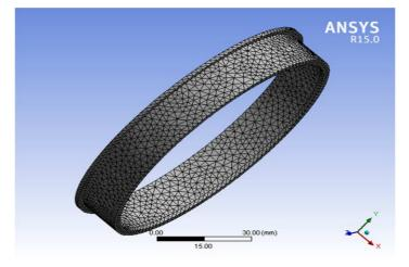
Fig. 6 – Fine meshing of cap
