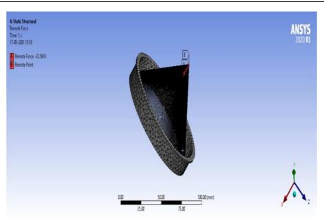
Fig. 7 – Remote force applied on the cap
