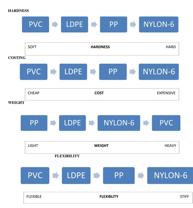
From charts, comparison of different materials with respect to various parameters is shown. To select theoptimum material for the cap all the parameters must meet the customer requirement. The cap material must withstand the stress induced due to force acting on the cap and at the same time it must be cost effective.
