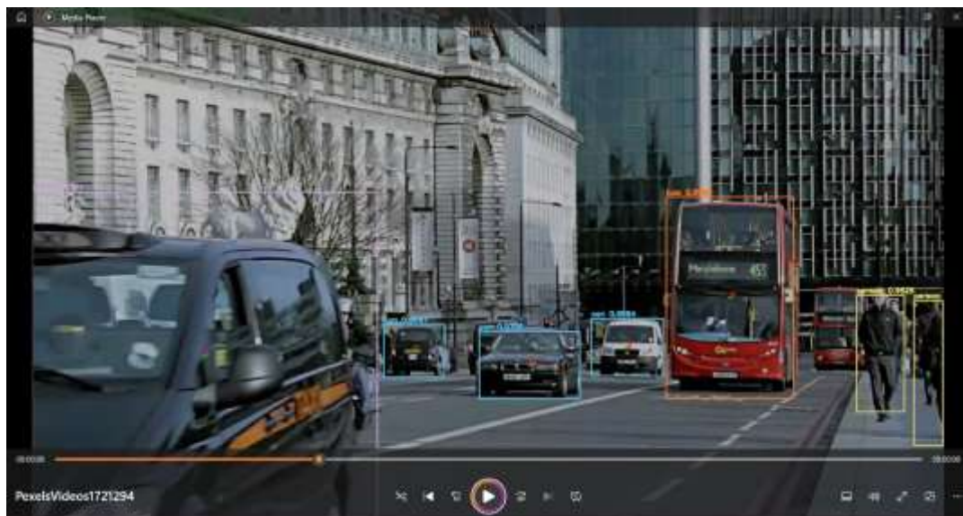
Figure 8: video frame with classification of persons, cars & buses with an accuracy of 94% ,96% & 99%
