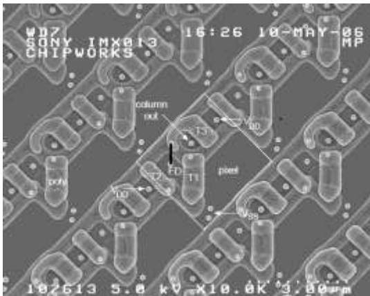
Fig. 6. Plan-View SEM of Pixels at the Polysilicon Level
